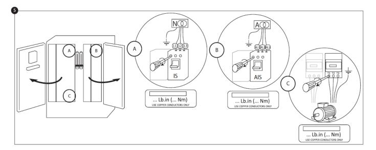
Connect the normal input power, the alternate input power and the motor on their respective terminals. Secure with the appropriate torque as indicated on the torque label and verify all connections.
