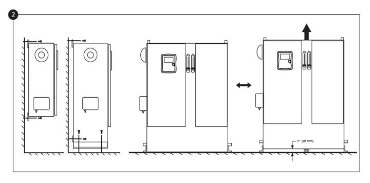
Verify that the controller is installed securely on the wall, or optionally on the mounting stand.
