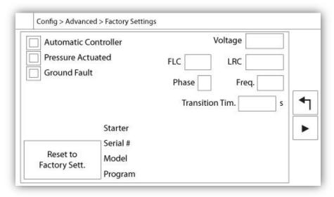
The factory settings are always pre-configured at the factory and set the main parameters of the controller. Most of the settings found on this page can only be changed by an authorized Tornatech employee and is protected by a level 8 password.
