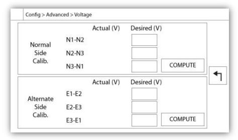
To calibrate the voltage sensing element of a power source, enter the 3 phase voltages as read on a calibrated meter then press compute. In the case of a transfer switch model, 3 additional voltages need to be calibrated the same way.
