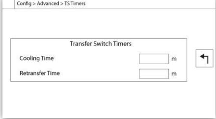
Most common timers for the transfer switch control can be configured here. Note that any timer set to 0 will remove the delay in the decision process.
