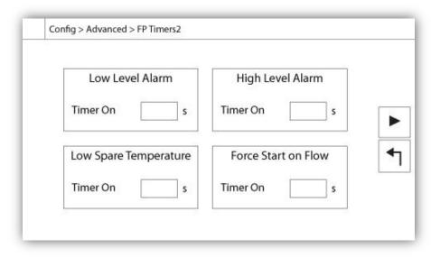
Most common timers can be configured here. Note that any timer set to 0 will remove the delay in the decision process.
