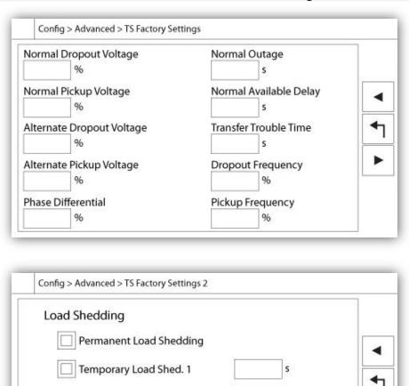
The factory settings are always pre-configured at the factory and set the main parameters of the controller. Most of the settings found on this page can only be changed by an authorized Tornatech employee and is protected by a level 8 password.
