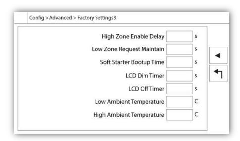
Higher Zone Enable Delay: Delay, in seconds, after which a motor run signal is sent to a higher zone controller. This option is only used for controllers in series.
