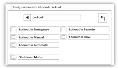
These pages allow to configure the Lockout input and the interlock output parameters. To be active, those options need to be assigned to an Input or an Output on the I/O board.
