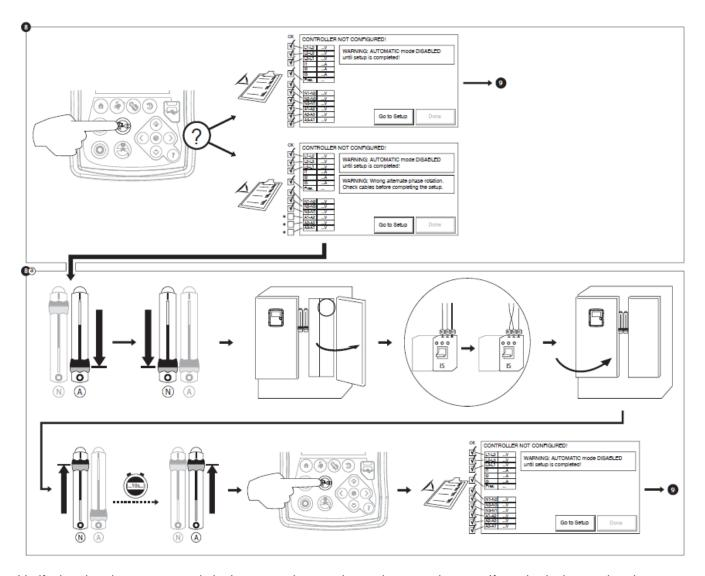
Verify that the alternate power is in the same phase order as the normal power. If required, change the alternate power wiring order to fit the one of the normal power.
