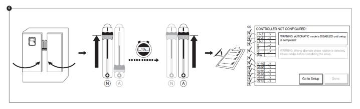
Secure the doors in the closed position then put the normal power circuit breaker disconnecting means in the ON position. Wait 10 seconds for the controller to load correctly, then put the alternate power circuit breaker disconnecting means to the ON position. Verify the readings on the controller main screen.
