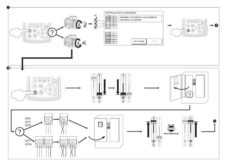
Verify the motor rotation to ensure that the pump is turning in the right direction. The START and STOP push buttons can be used to toggle the motor ON/OFF.
