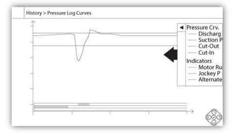
The vertical axis represents the pressure in the actual unit selected. Its scale is dynamic and will resize depending on the highest recorded value. The horizontal axis represents time and period. The left part of the horizontal axis shows the beginning of the current scope and the right part shows the end of the scope. Located just right of the
