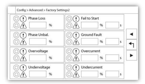
Phase Loss: Sets the value in percentage of the nominal voltage. If a phase voltage reading is lower, the corresponding alarm/warning will be activated.
