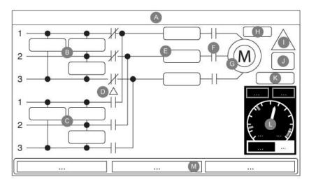
The home page displays all controller statuses and important values of the controller. All voltages, currents, pressure, motor state and status, as well as all timers and motor starting sequences.
